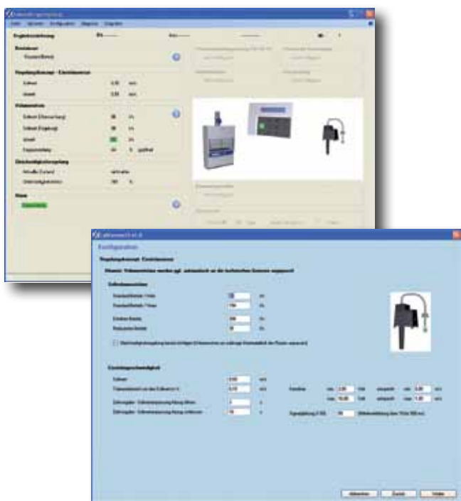
Dialogue for fume cupboard control with face velocity transducer
