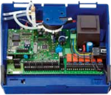
EASYLAB controller with expansion modules
